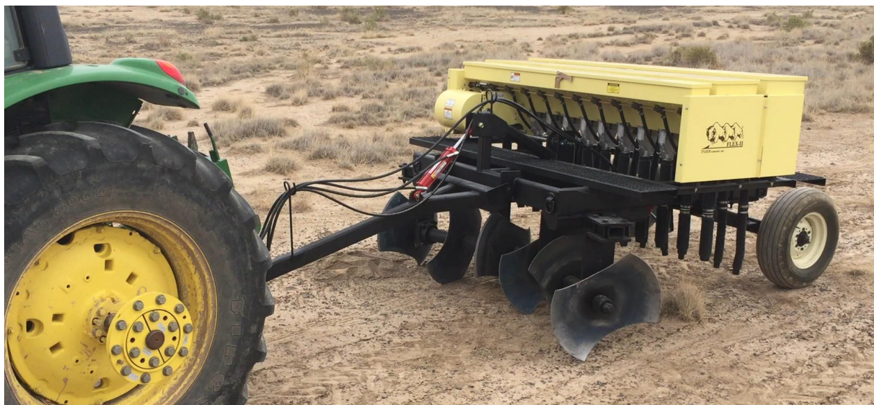
Figure 7. Pothole seeder. When the discs are dragged, the large notches produces a pattern of mounds and holes. The seeder requires a tractor of at least 50 HP with two sets of hydraulic ports.
