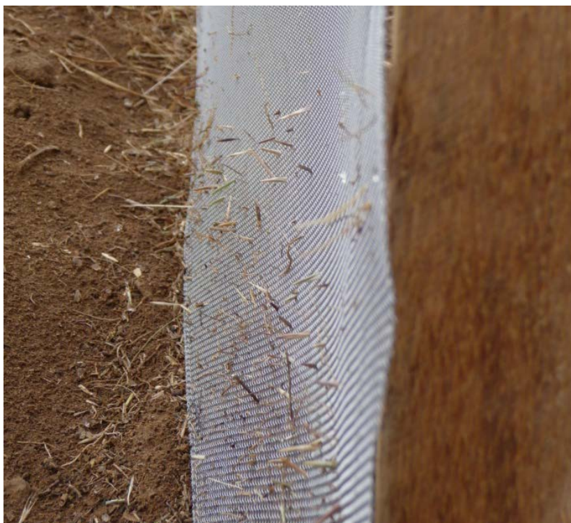
Figure Gulley 6. Cheatgrass seeds caught in aluminum window screen barrier.
