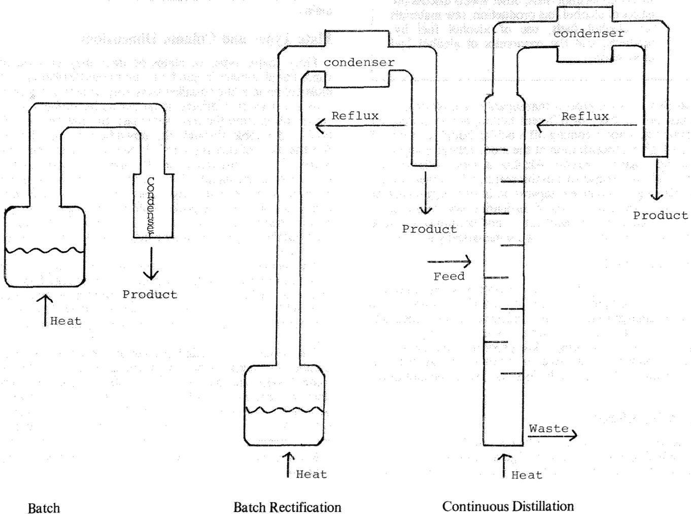
Figure 1: Types of distillation systems.
