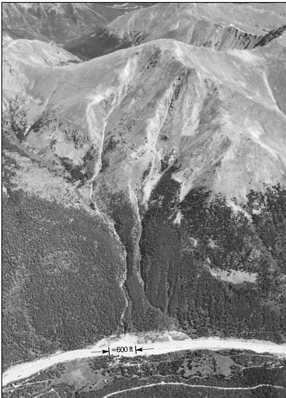
Debris flow source area, scoured channel and natural levees, vicinity of Arapahoe Basin PHOTO BY JEFF COE, USGS
